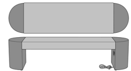
Tarragona Bench, 60" Seat Width, with Fusion Top, with Power Module on Left Side Model: TGNABNB11PG1L 80.5W 20.5D 19H
